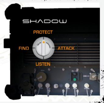
as a function of the interference waveforms, as well as of the threats it identifies, from its ability to detect and classify them. The system only transmits in the presence of a threat and automatically reconfigures itself depending on its location. Compared with traditional systems, this adaptability considerably reduces operators' and vehicle passengers' exposure to radiation; which makes the system especially well suited to intensive use. Bull said
