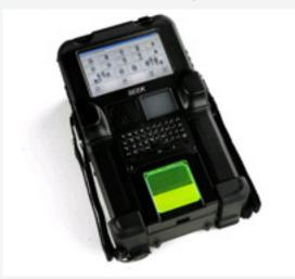
formation. The device is called a Secure Electronic Enrollment Kit, or SEEK, a handheld biometrics recorder that takes iris scans, fingerprints and facial scans and ports them back to an FBI database in West Virginia in
