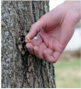
Missouri S&T researchers use a device called a solid-phase microextraction fiber, or SPME, to detect traces of chemicals at minute levels in trees.
