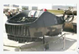
Urban Aeronautics is developing an unmanned vehicle powered by internal lift fans, the prototype has been flying since 2009 and will soon demonstrate hovering and flying at low altitude, controlled by the autonomous flight control and navigation system. Photo: Noam Eshell Defense Update
