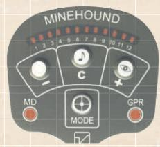
A push button in the handle allows the operator to select the operation mode MD or GPR or both.
