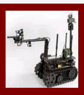
QinetiQ North America offers modular CBRNE (chemical, biological, radiological, nuclear, explosive) kits as an addition to new or existing models of the TALON robot.
