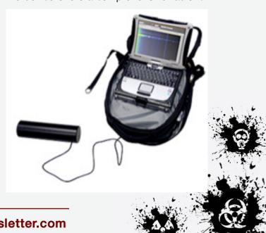
clide database for reference. All measured data can be compared to the known spectrums for very specific analysis.
