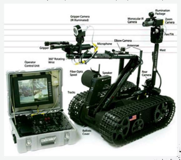
coded according to intensity. As the robot navigates in the environment, a breadcrumb-like trail is generated and displayed on the operator control unit. The system is self-contained and has the ability to work with a variety of radiation sensors," Stricker said
