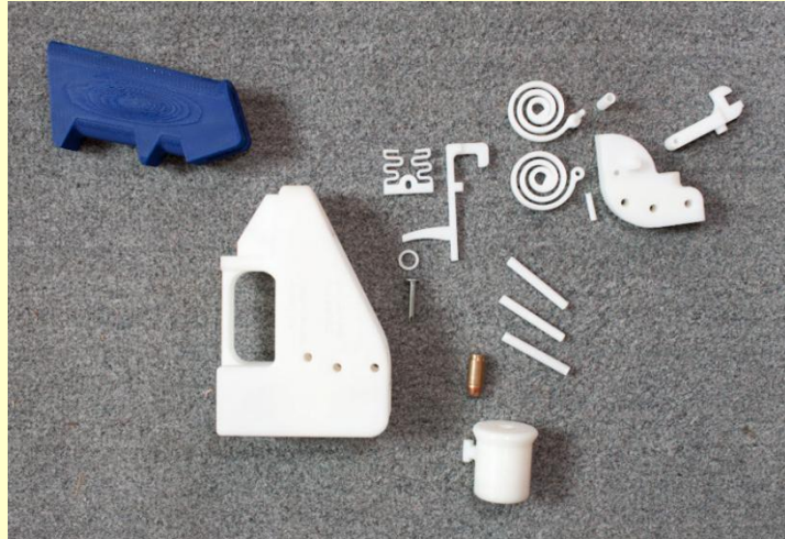
The sixteen pieces of Defense Distributed's printed handgun, including spiral springs for its hammer mechanism and a nail used as its firing pin. (Credit: Michael Thad Carter for Forbes)
