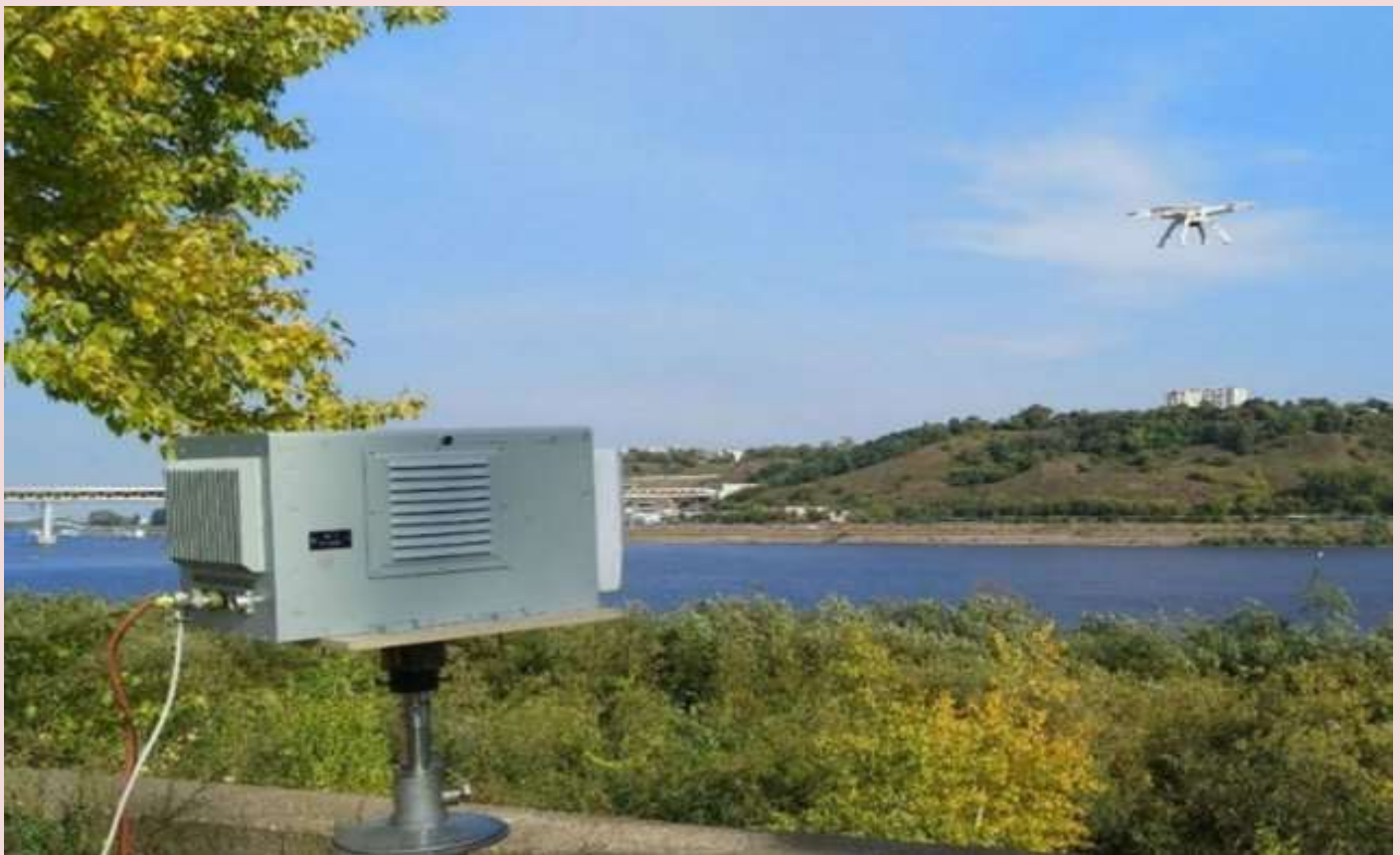
Radar developed to detect tiny drones (image: Ruselectronics)
