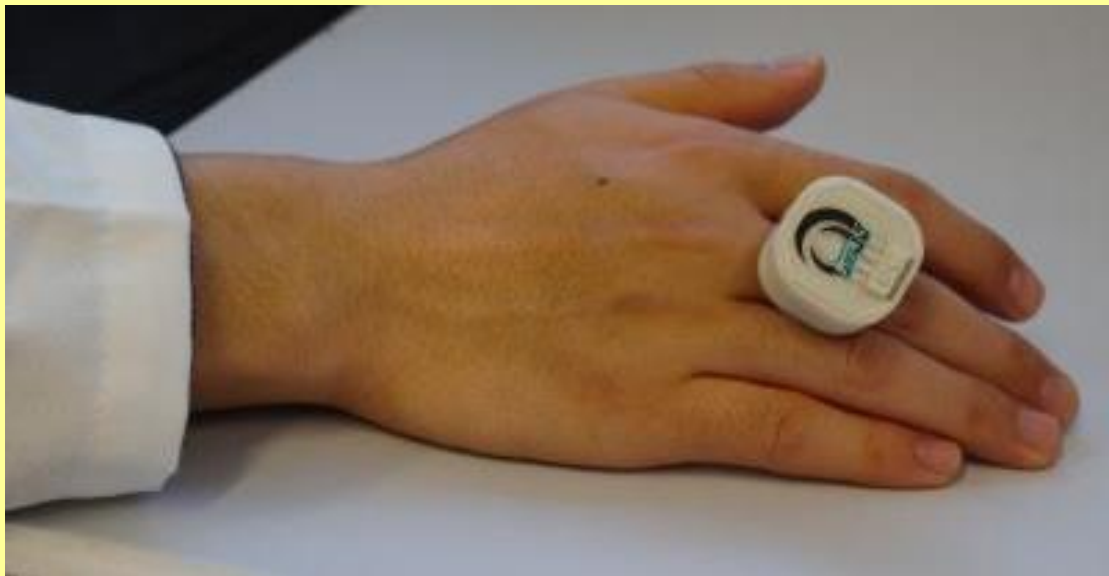
A first-of-its kind ring sensor can detect chemical and biological threats. American Chemical Society
