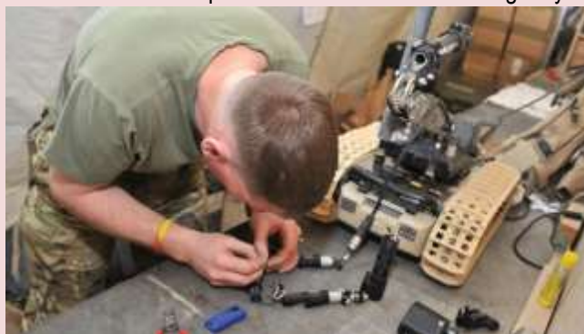
An REME corporal repairing a Dragon Runner EOD variant © Crown 2012
