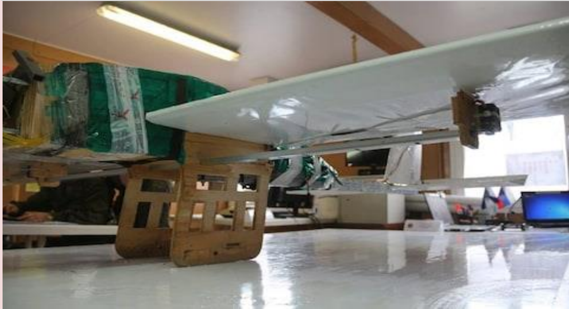
The drones appear to be made partly of wood and held together by masking tape Credit: Russian Ministry of Defence
