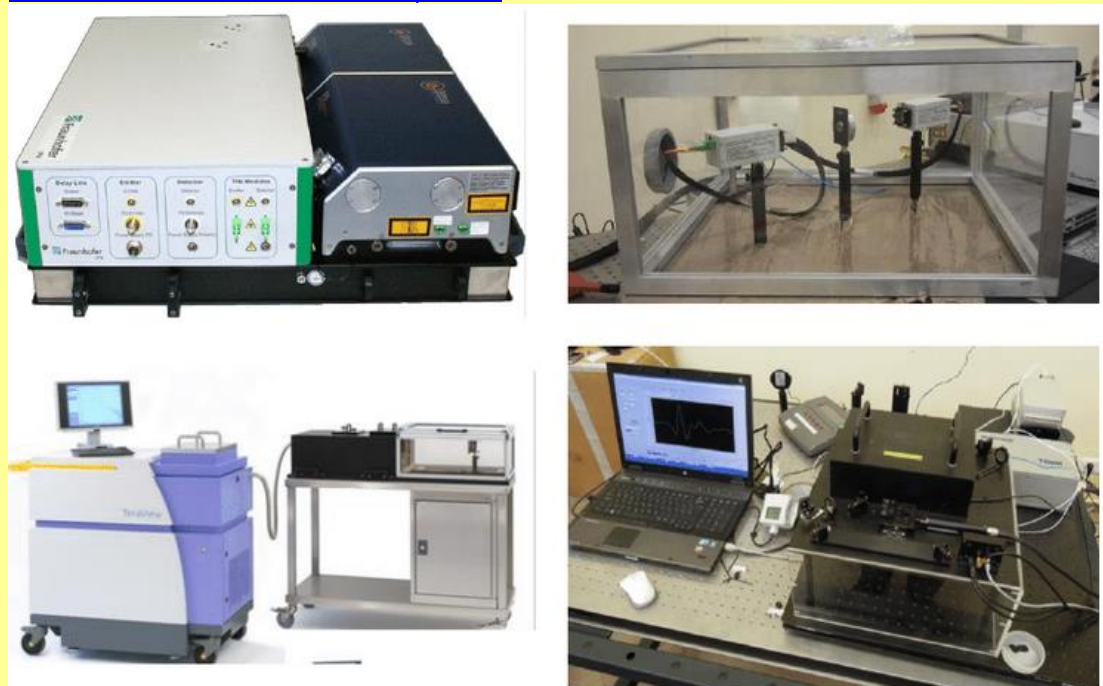
Figure 1. The photonic THz systems used in this trial. Top left: Optical subsystem of the NorT spectrometer; top right: fiber-coupled NorT measurement heads in dried air enclosure; bottom left: TPS Spectra 3000 with external fiber-coupled add-on compartment for reflection measurements; bottom right: modified electro-optic TeraKit spectrometer.
