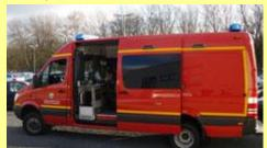
for the fast and reliable detecting of radiological and chemical contamination. The measuring equipment is housed in the crew cabinet with an autonomous power supply. This computer-operated system enables the collection, evaluation and storage of each pollution load including the relevant geographical coordinates. Data is transmitted to higher echelon elements via the GSM network. As an option, additional equipment is available for
