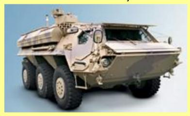
Packed with built-in state-of-the-art detection equipment, Rheinmetall Defence's Fuchs/Fox armoured NBC reconnaissance system can quickly determine the presence of nuclear, biological and chemical contamination on the ground and in the air, covering large areas. Rugged and reliable, this amphibious, all-terrain armoured vehicle is able to conduct its mission even in the toughest terrain. Nearly 300
