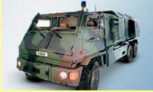
The Bio-Spür-Fuchs and Bio-Spür-Yak are both highly mobile reconnaissance systems capable of detecting the presence of weaponized biological agents and contaminants in the air, on the ground and in water, quickly covering large areas. For the first time, these two highly integrated systems make it possible to search for biological threats.
