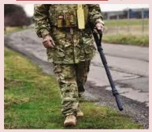
to EOD Marines in the fourth quarter of 2019, the wire detector includes a one-piece foldable design that is lighter and more time-efficient than the previous systems.
