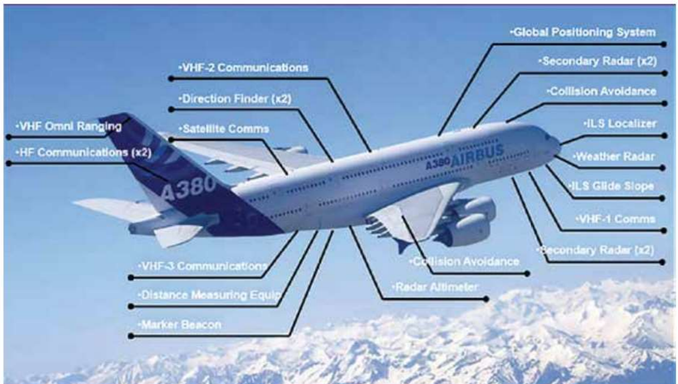
Figure 1.7. Airbus A-380 electronic systems. (Source: FAA.)
