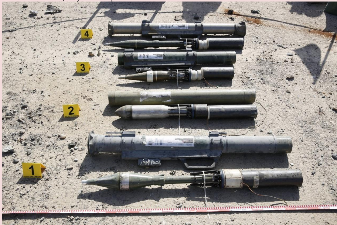
A series of shoulder-fired, recoilless launchers made by the Islamic State, shown with a variety of repurposed projectiles. ISIS weapons engineers took Soviet-era munitions and made Western-style disposable launchers for them, even affixing written instructions for their use. Credit Damien Spleeters/Conflict Armament Research
