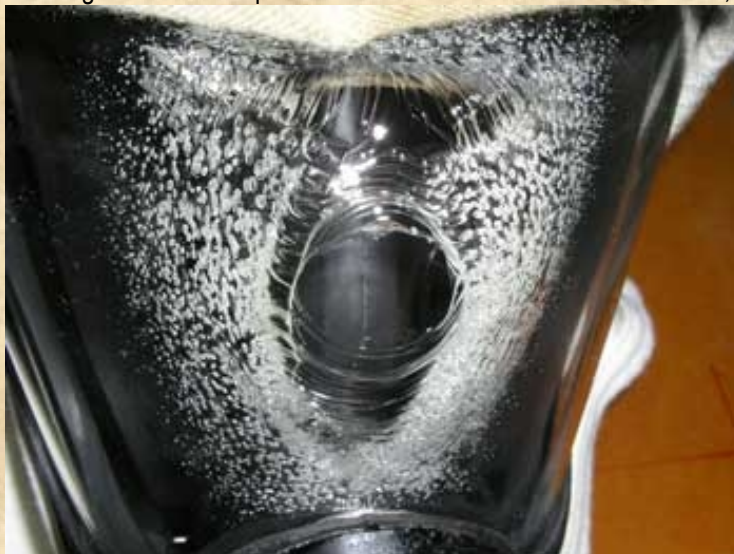
Typical fire-fighter breathing apparatus damaged in NIST tests shows facepiece warping under high heats.
