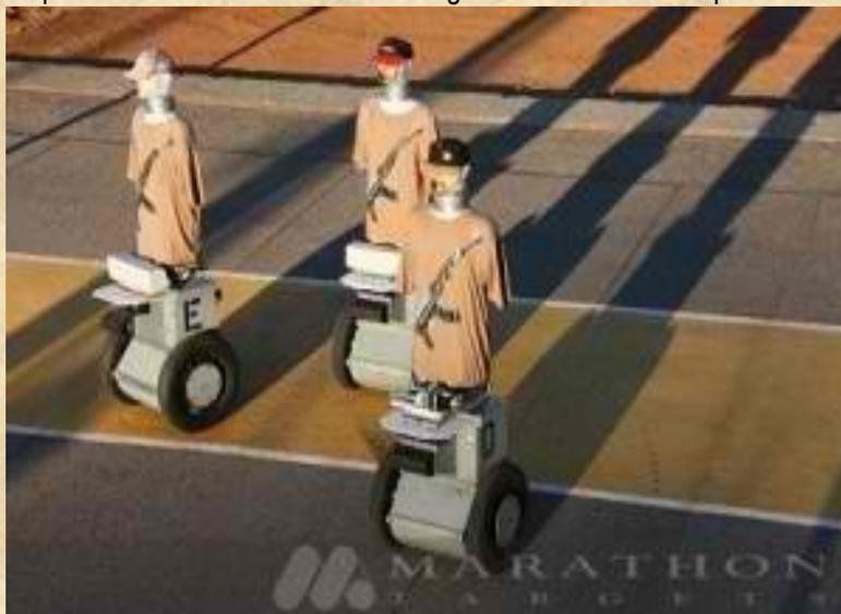
than the armored mechanism carrying it. The time needed to recharge the battery has been reduced from eight hours to 2.5 hours, and it can operate at higher temperature ranges. Finally, replaceable external speakers allow it to “talk” or emit simulated gunshots.
