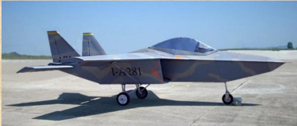
Single-seated, ultra light (weights 200kg) with an engine of 46hp.
