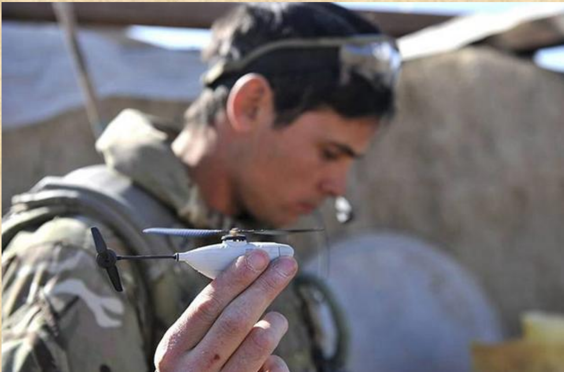
Black Hornet measures around 4 inches by 1 inch and weighs 16 grams; and is designed to provide troops with situational awareness via a micro camera that delivers full motion video and still images. Images are displayed on a handheld terminal, giving troops the ability to see around corners, over walls and other battlefield obstacles. The system is capable of performing in harsh environments and windy conditions. The UK MoD has acquired the system from Prox Dynamics of
