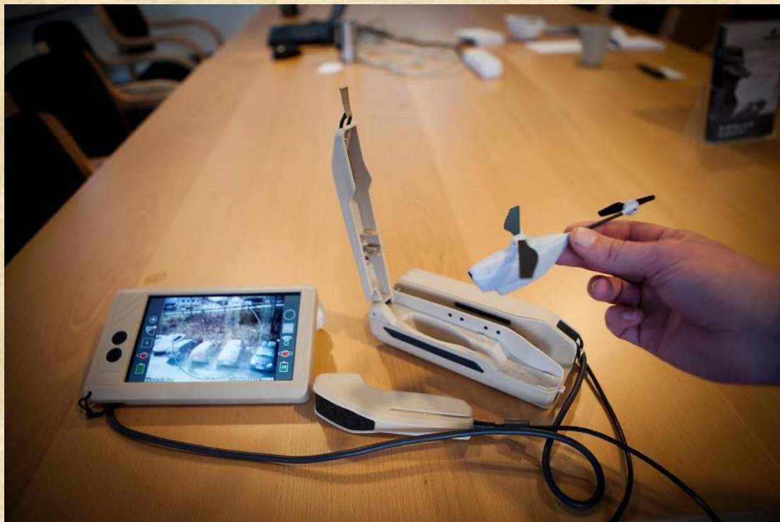
Black Hornet measures around 4 inches by 1 inch and weighs 16 grams; and is designed to provide troops with situational awareness via a micro camera that delivers full motion video and still images. Images are displayed on a handheld terminal, giving troops the ability to see around corners, over walls and other battlefield obstacles. The system is capable of performing in harsh environments and windy conditions. The UK MoD has acquired the system from Prox Dynamics of
