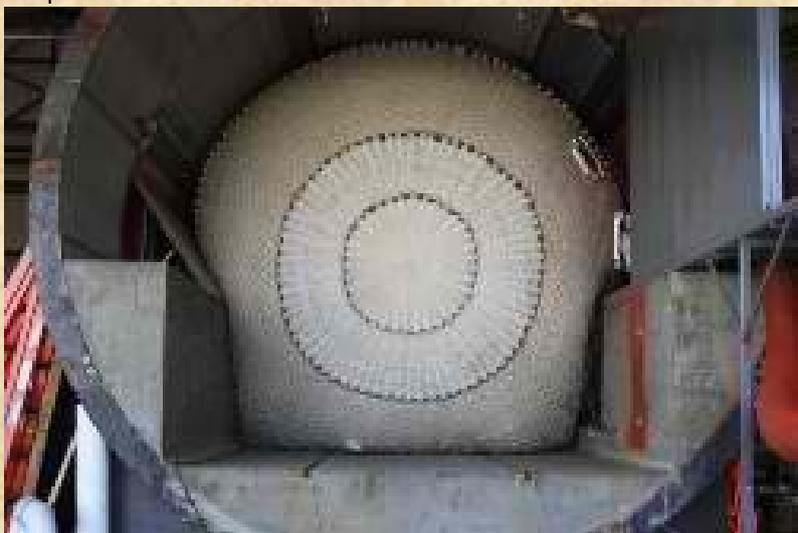
prototype failed during pressurized testing. S&T's project team aggressively pursued new designs, ultimately settling on the present one: three separate layers.
