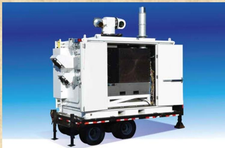
of tests against representative airborne targets. Lockheed Martin developed the Area Defense Anti-Munitions (ADAM) system to provide a defense against short-range threats, such as rockets and unmanned aerial systems.
