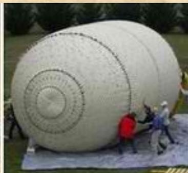
Inflatable plugs being developed with funding from DHS, could have saved some of New York's subway and highway tunnels from flooding during Hurricane Sandy, according to the developers of the plugs.
