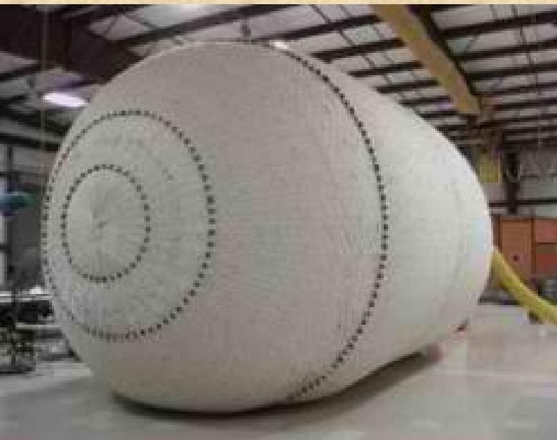
seal off a section of tunnel before flooding gets out of control.
