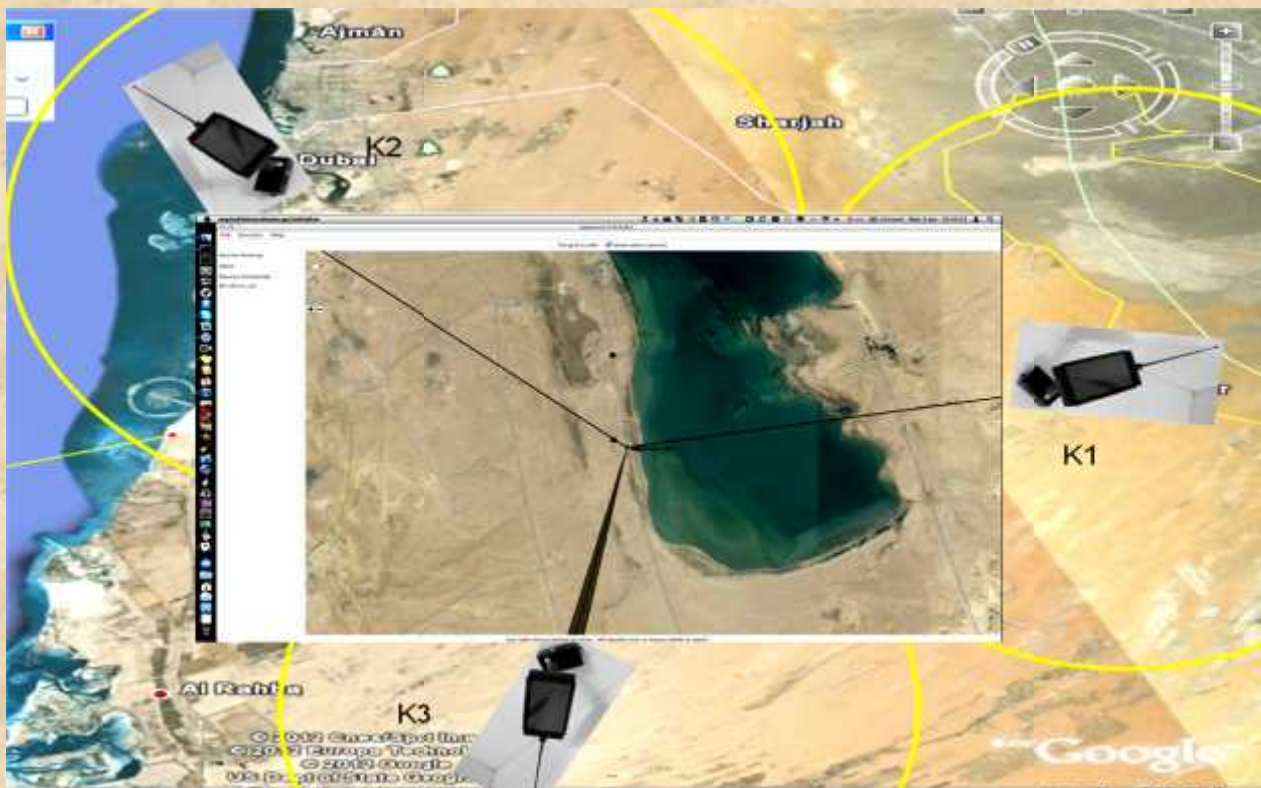
DRAMS system using 3 KYKLOTRON E sensors (k1,- 2,-3) for 360 degrees protection area. At the center of figure, a vision of the DRAMS controller computer screen. Controller is shown and the three lines – antennas of K1-K2-K3 sensors users (black lines) on screen. Controller coordinates and controls the 3 users of the system.
