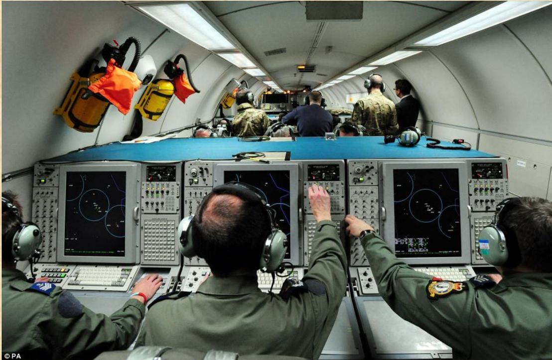
Control centre: The normal 18 man crew comprises four flight-deck crew, three technicians and an 11-man mission crew. The mission crew comprises a tactical director, a fighter allocator, three weapons controllers, a surveillance controller, two surveillance operators, a data-link manager, a communications
