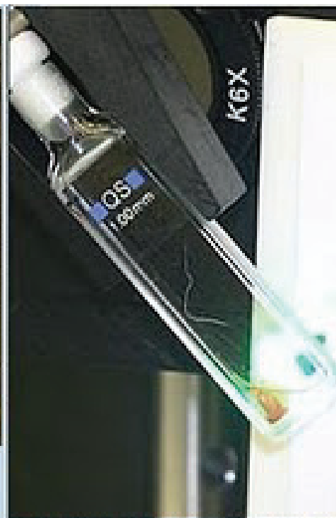
Ultraviolet light breaks down a chemical agent inside a quartz cuvette. The brown material is the decomposition byproduct.
