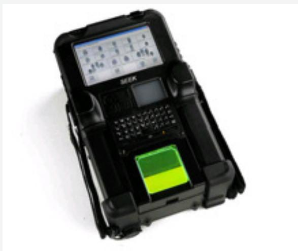
formation. The device is called a Secure Electronic Enrollment Kit, or SEEK, a handheld biometrics recorder that takes iris scans, fingerprints and facial scans and ports them back to an FBI database in West Virginia in seconds.
