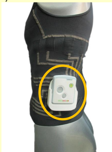
On the side of the hWear shirt, snaps hold the telemetry unit (photo).
