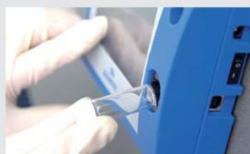
1. Start test by determining the background value of cuvette
