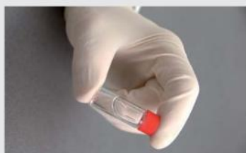
5. Dissolve substrate in cap by gently shaking the cuvette
