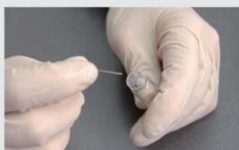
2. Take blood sample and add glass capillary to cuvette
