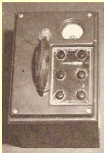
A radiation survey device of the sort produced during World War II by the Victoreen Instrument Company in Cleveland, in collaboration with the University of Chicago scientists.
