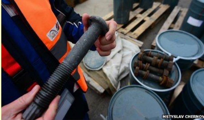
Bolts used to assemble the Arch are some 15cm long and weigh more than 1kg
