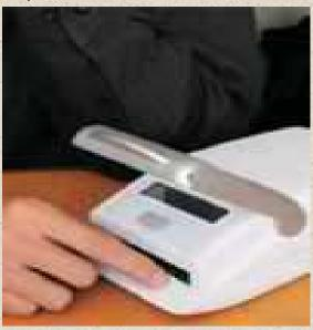
co-founded in 2004. (The company has recently been named by MIT's Technology Review as one of the 50 most innovative companies in the world.) The microchip inside the device is formed through injection molding and holds miniature forms of test tubes and chemicals; the cost of the chip is about \$1 and the entire instrument about \$100.
