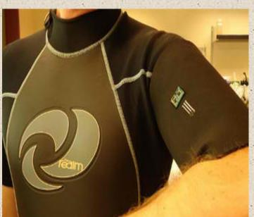
Flexible sensors printed on neoprene wetsuit sleeve // Source: calit2.net
