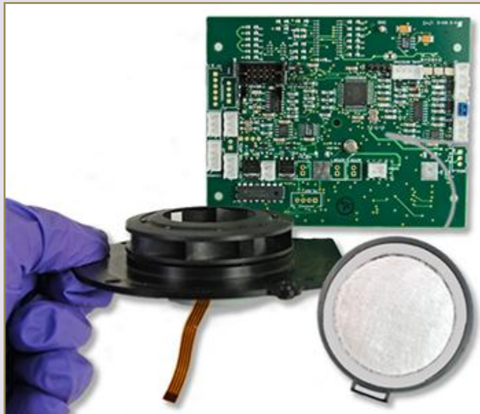
Figure 2: 300 liter/minute aerosol sample collector components.
