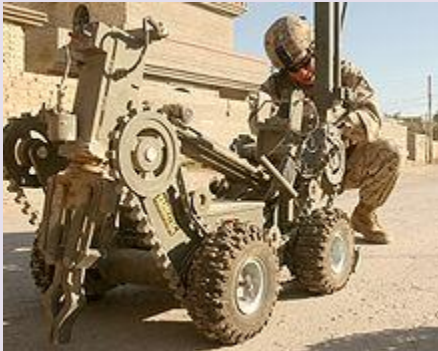
A U.S. Marine Corps technician prepares to use a telerobot to detonate a buried improvised explosive device near Camp Fallujah, Iraq
