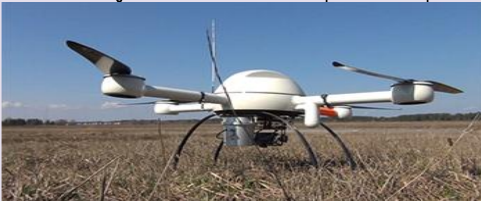
Figure 3: Radiation detector subsystem shown in a previous application, mounted in a cylindrical enclosure to the underside of a miniature UAV helicopter.
