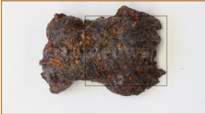
Rusty warhead fragment. Consists of a layer of alloyed steel. Strongly deformed and folded. (picture Jeroen Akkermans / RTL News).
