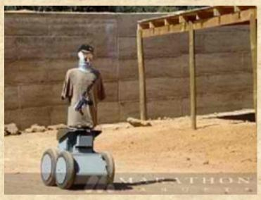
"The Marathon targets used in the comparative test had two wheels and required a flat, level surface to operate," said a subject matter expert from the Marine Corps. "This was not practical for use on Marine Corps ranges
