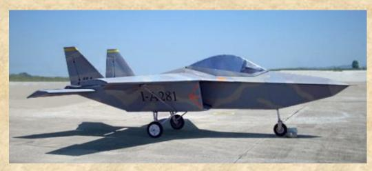
Single-seated, ultra light (weights 200kg) with an engine of 46hp.
