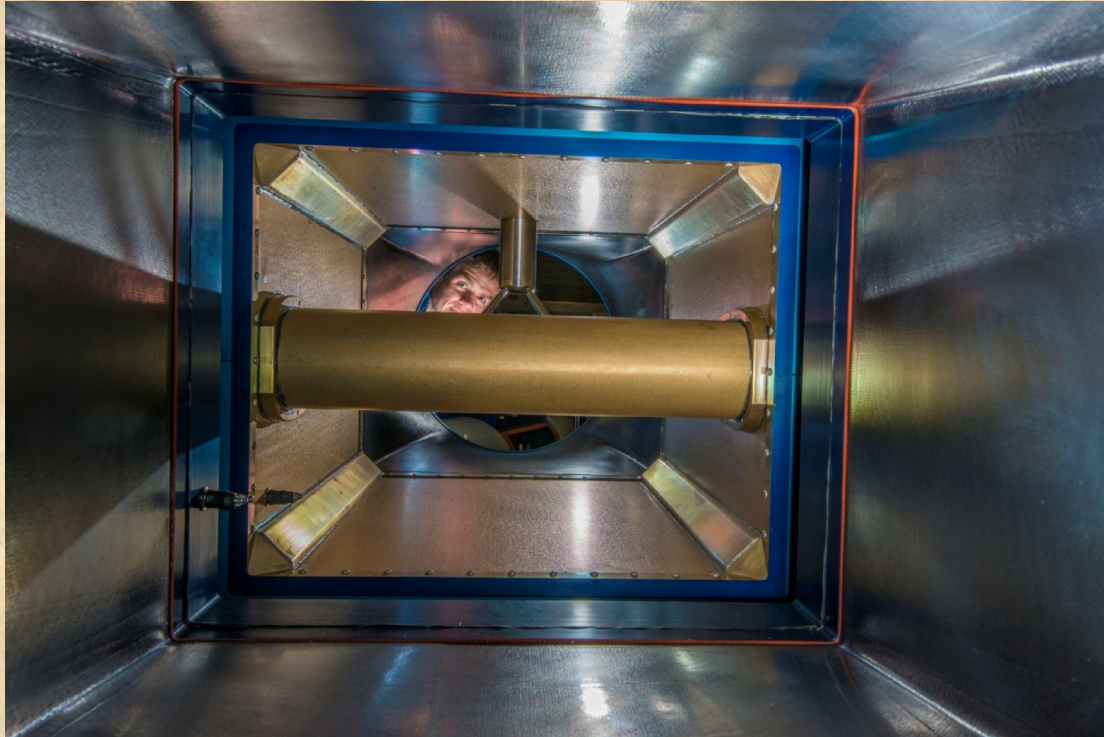
A researcher checks air flow in the Harvester particulate sampling pod. (Photo by Randy Montoya)
