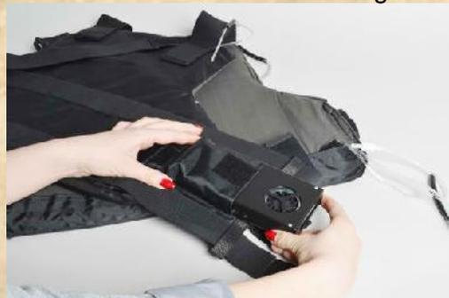
built into the vest; so EMPA engineers designed a miniaturized version themselves. Two units including batteries and control electronics now provide the cooling air circulation in the vest.
