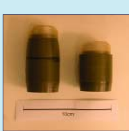
Medium calibre variants (of different mass and aerodynamic properties) of 37 mm DIP concepts, showing the carrier body and irritant payload in the nose, within a frangible cap.
