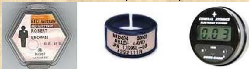
Dosimeters: film badge (left), ring badge (center), and real-time (right). (Source: OSHA and U.S.D.H.S.)
